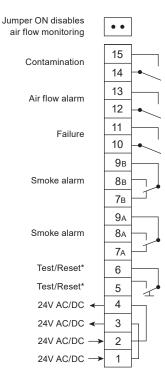
The relay outputs are shown in power off/alarm condition.
