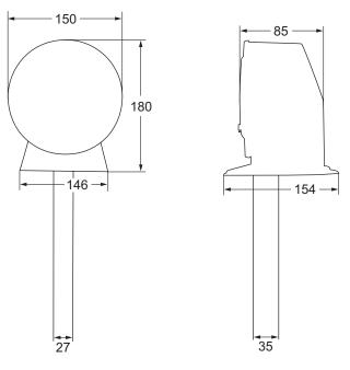
The analogue smoke detector controls the alarm signals from smoke in it's chamber by measuring time, amplitude of signal and signal spread. Before transmitting a fire signal the smoke value must conform with preset data.
