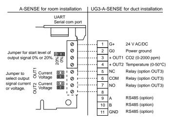
\* In the duct mounted version (UG3-A-SENSE), the temperature accuracy is dependent of the ambient temperature by the UG3-A-SENSE. In case of big temperature difference inside and outside the duct, the accuracy can be more than ±1°C. Note that the temperature measurement function requires air flow in the duct.
