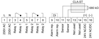
The relay outputs are shown in alarm/no power on condition. Max 5A, 250V
