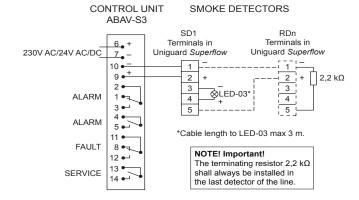
The alarm relay and the failure relay outputs are shown in alarm/no power on condition and the service alarm relay is shown in operative/no power on condition.
