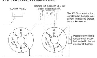
The base is provided with a resistor, 330 Ohm, which will limit the current in the loop to different models of fire alarm panels. The 330 Ohm resistor should not be taken away.
